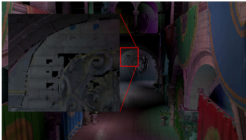
Figure 11 – Screenshot showing how the final render of the visibility buffer renderer artefacts appears at run-time. The artefacts are mainly located at the intersection of two different materials in screen space due to the nature of their origin, as explained in Section 5.3.
